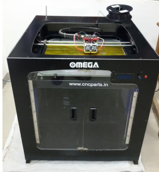
**Fig. 1.** FDM based 3D printer
