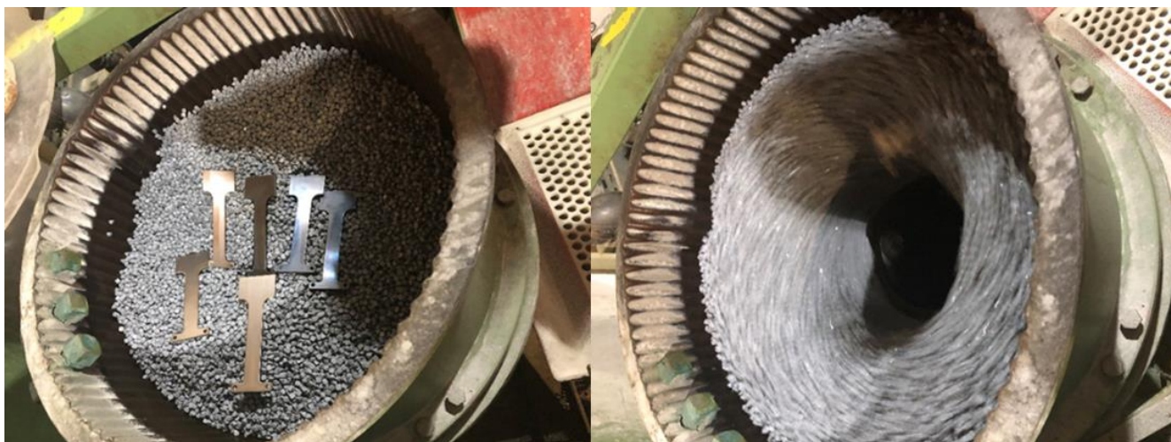
Figure 9. Installation for centrifugal hardening treatment (Rosler)
