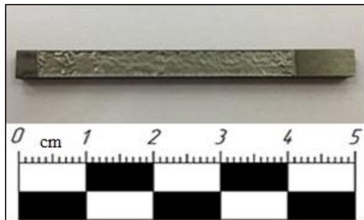
Figure 6. Sample of the iron-chromium-nickel alloy after etching
