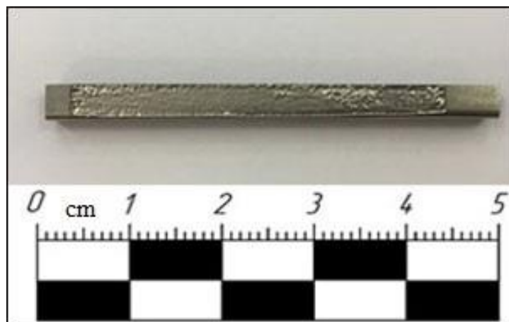
Figure 5. Sample of the titanium alloy after etching
