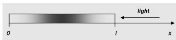
Figure 2. Solid cylindrical bar with adiabatic lateral walls
