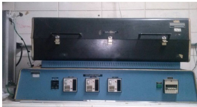
Figure 1. Picture of the furnace device used in the synthesis of the CuNbGaSe 3 compound
