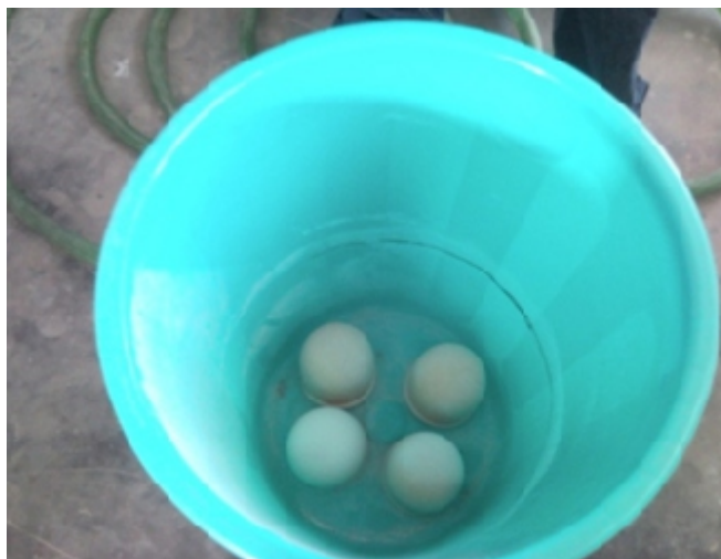
Figura 2. Photograph of the inside of the filter with four ceramic cartridges (without the AA)
