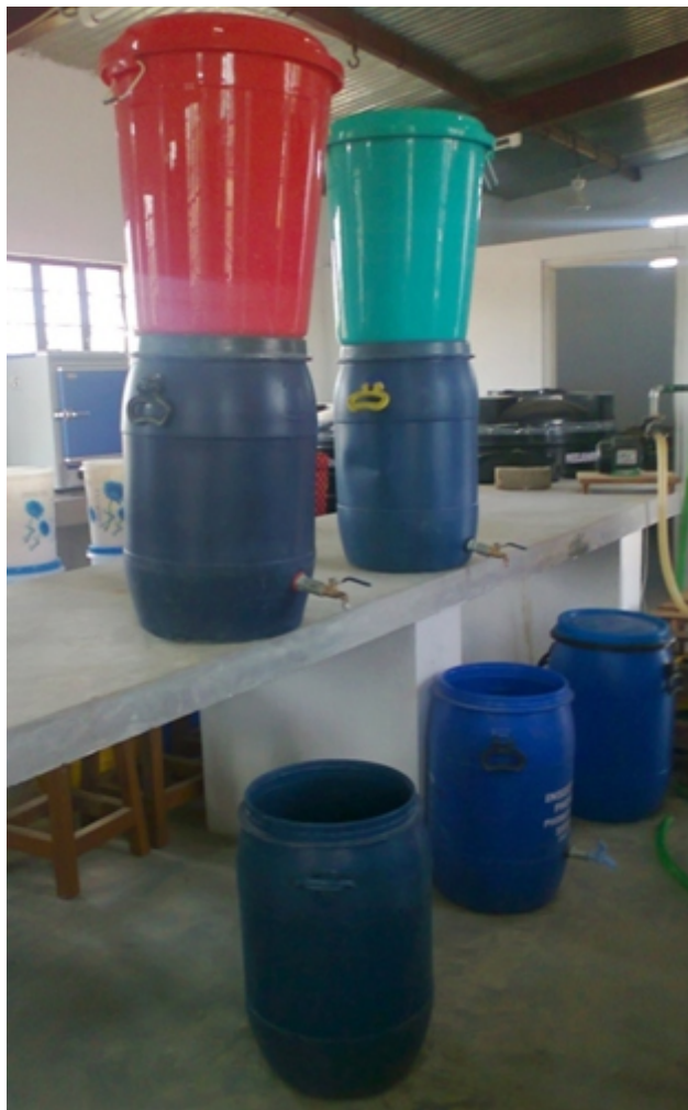
Figura 3. Photo of the fabricated filter with four ceramic candles with Activated Alumina
