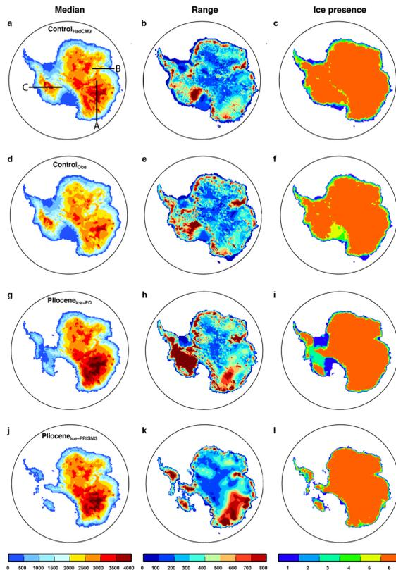
**Figure 7.** Median, range and coverages of ice thickness from the six ISM simulations. From top to bottom shows the four experiments. All six ice thickness values for each location are sorted, the median is shown as the mean of the 3th and 4th value (in m), the range is the difference between the 6th and the 1st, divided by two and ice coverage counts if any ice is present. The black lines in **(a)** represent the cross sections: A – Wilkes basin, B – Lambert ice stream and C – the WAIS.
