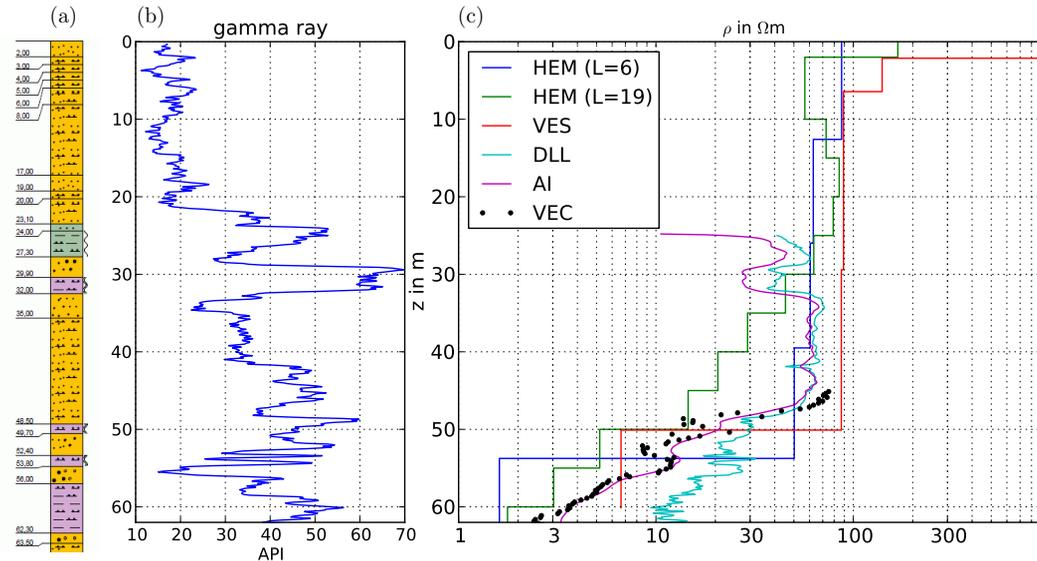
**Fig. 2.** Lithology (a), gamma ray (b) and resistivity information (c) at the CLIWAT 2 borehole: 6- and 19-layer HEM solution, VES model, dual laterolog, induction log and vertical electric chain.
