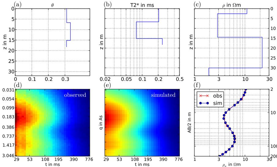
**Fig. 5.** Result of independent inversions (subplots as in Fig. 3) of the MRS and VES soundings for the location SKD using 3 and 4 layers, respectively.
