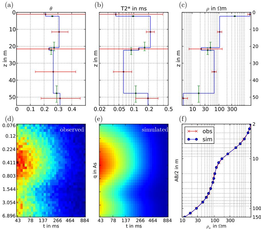
**Fig. 3.** Joint inversion result of the MRS and VES soundings at the CLIWAT 2 borehole: water content (a) decay time (b) and resistivity (c) as a function of depth including uncertainty, MRS data cube observed (d) and simulated (e), and measured/modelled apparent resistivity (f).
