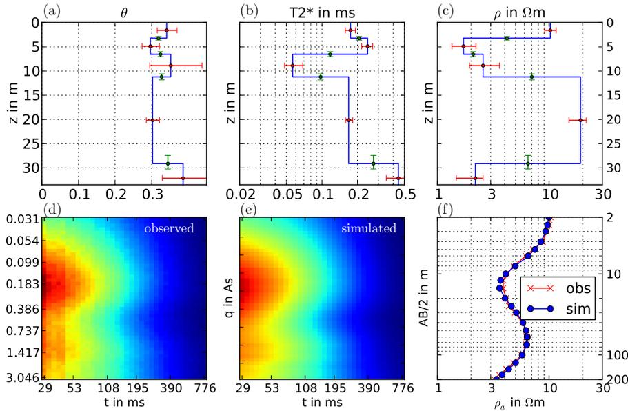
**Fig. 6.** Joint inversion result (subplots as in Fig. 3) of the MRS and VES soundings for the location SKD.
