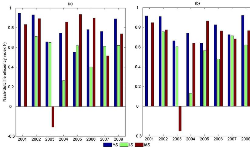
**Fig. 3.** Nash-Sutcliffe efficiency for seasonal simulations with **(a)** Model I and **(b)** Model II. AET modeled with  $\Delta t = 30$  min.
