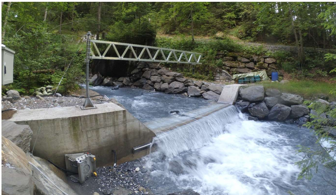
Figure S50. Automatic picture of the Avançon de Nant measurement station at the Vallon de Nant outlet on July 30 th 2018. The river stage measure by the SONAR above the middle point of the river is disturbed by a rock.
