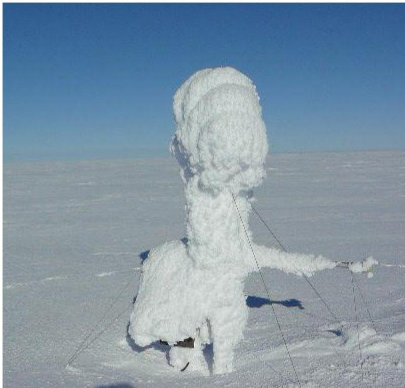
**Figure 21.** A photo of an Automatic Weather Station covered by thick rime ice at Roosevelt Island ( $79^{\circ}25'$  S,  $162^{\circ}00'$  W), 23<sup>rd</sup> October, 2011. Photo provided by N. Bertler.
