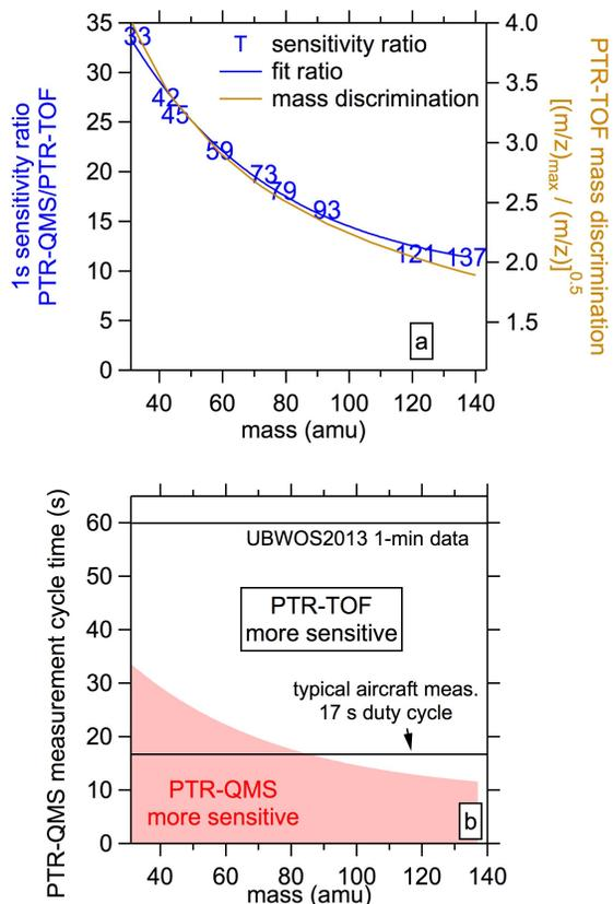
**Figure 4.** (a) The ratio of the 1 s sensitivities of PTR-QMS/PTR-TOF together with the PTR-TOF mass discrimination. (b) A mass dependent curve showing the length of the PTR-QMS measurement cycle, where the PTR-QMS is as sensitive as the PTR-TOF (identical to the fit in a). In aircraft measurements a duty cycle of 17 s is typical (PTR-TOF more sensitive above mass 80) and at ground sites 1 min measurements are typical (PTR-TOF more sensitive for all masses).
