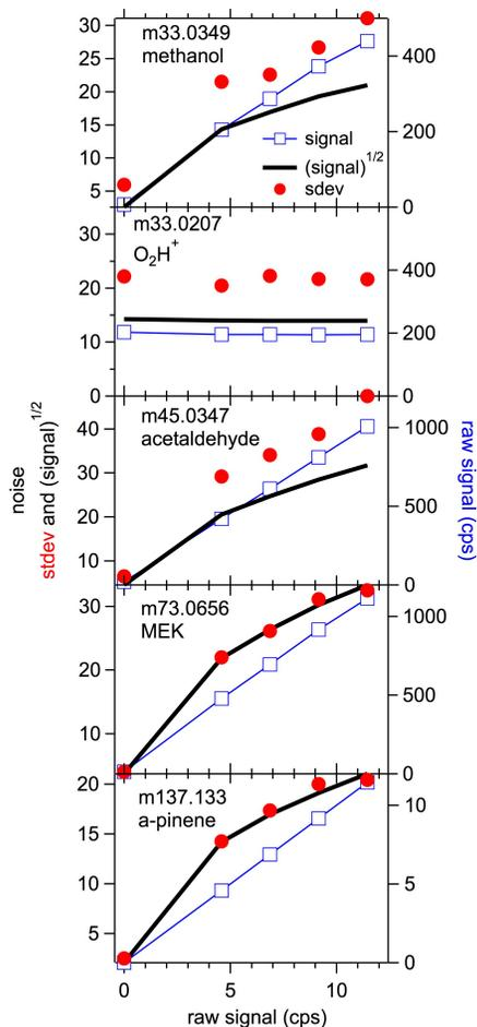
**Figure 5.** Signal,  $(\text{signal})^{1/2}$ , and standard deviation of the signal (noise) during a typical PTR-TOF calibration measurement for some selected masses.
