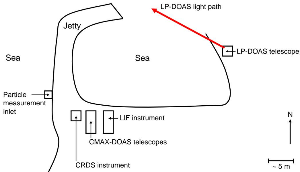
**Fig. 2.** A schematic of the Roscoff measurement site at high tide. Highlighted instrumentation includes LIF, LP-DOAS, Concurrent Multi Axis DOAS (CMAS-DOAS), Cavity Ringdown Spectroscopy (CRDS) and particle number and size-distribution measurements.
