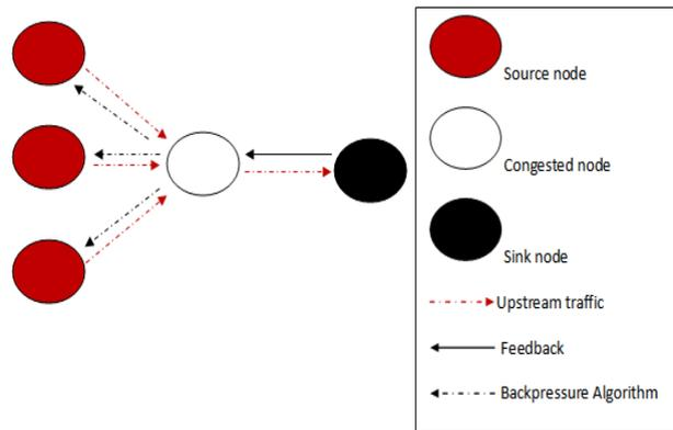
Figure 4: DelStatic Traffic Reduction Scenario
