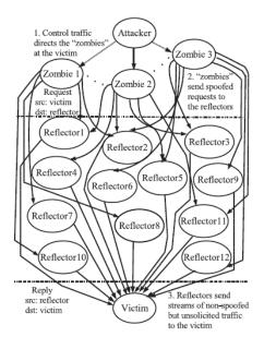
Figure 1. The structure of a distributed reflector denial of service (DRDoS) attack [7]
