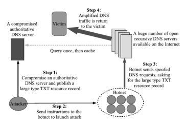
Figure 2. An example of a DNS amplification attack [4]
