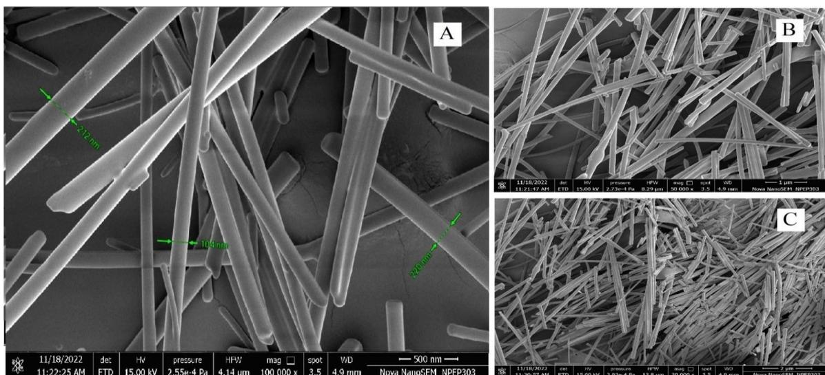
**Figure 2:** FE SEM Images of Drug Loaded Nanofibers at different magnifications: A. 100,000 X B. 50,000 X C. 30,000 X
