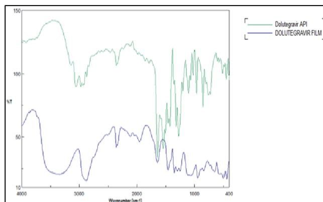
**Figure 6:** Overlay of FT IR spectra of dolutegravir and Nanofiber loaded film.
