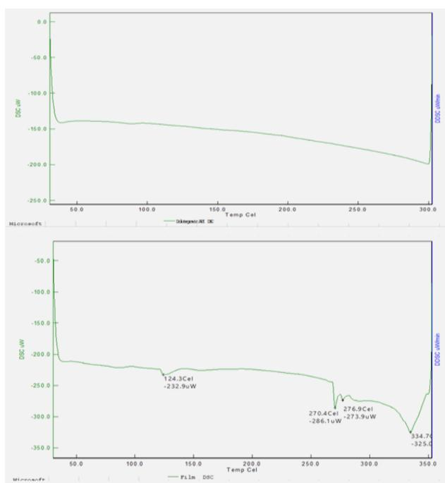
**Figure 7:** DSC Thermograph of Dolutegravir
