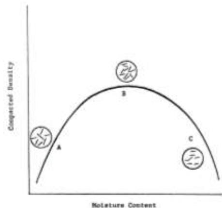
Fig. 7: Variation of compacted density with moisture content.
