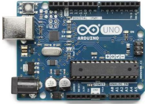
Figure 6. Data acquisition system, Arduino Uno
