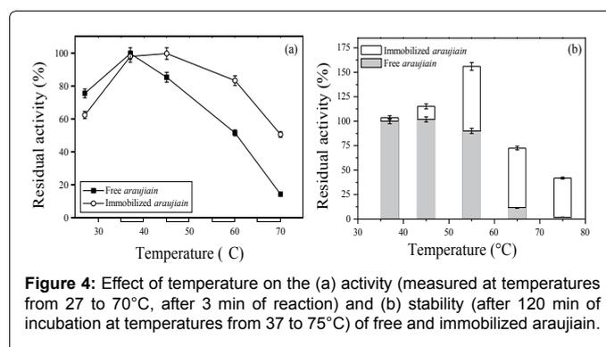
Figure 4: Effect of temperature on the (a) activity (measured at temperatures from 27 to 70°C, after 3 min of reaction) and (b) stability (after 120 min of incubation at temperatures from 37 to 75°C) of free and immobilized *araujiain*.
