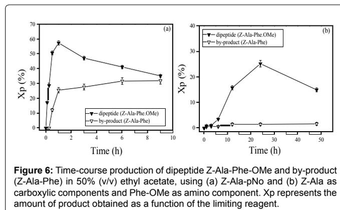
Figure 6: Time-course production of dipeptide Z-Ala-Phe-OMe and by-product (Z-Ala-Phe) in 50% (v/v) ethyl acetate, using (a) Z-Ala-pNo and (b) Z-Ala as carboxylic components and Phe-OMe as amino component. Xp represents the amount of product obtained as a function of the limiting reagent.
