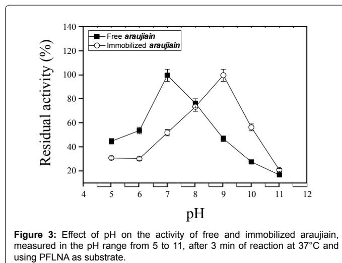
Figure 3: Effect of pH on the activity of free and immobilized *araujiain*, measured in the pH range from 5 to 11, after 3 min of reaction at 37°C and using PFLNA as substrate.
