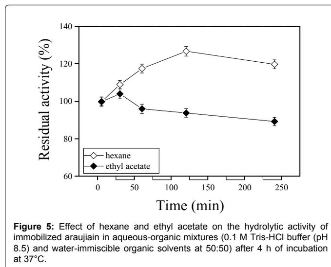
Figure 5: Effect of hexane and ethyl acetate on the hydrolytic activity of immobilized *araujiain* in aqueous-organic mixtures (0.1 M Tris-HCl buffer (pH 8.5) and water-immiscible organic solvents at 50:50) after 4 h of incubation at 37°C.
