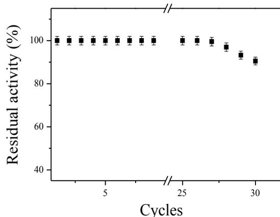
**Figure 2:** Residual activity (%) of immobilized *araujiain* after thirty cycles of the hydrolytic reaction. Each cycle was defined as the number of enzymatic reactions carried out during 3 min at 37°C and using PFLNA as substrate.
