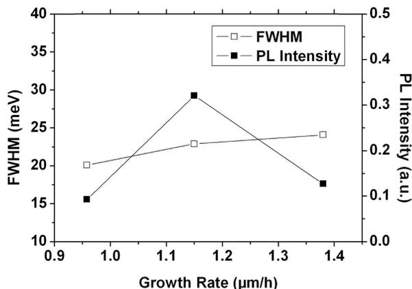
Fig. 6. PL FWHM and intensity of samples prepared at different growth rates.
