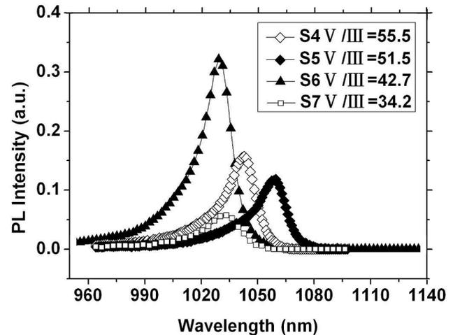
Fig. 3. PL spectra of samples grown at different V/III ratios.
