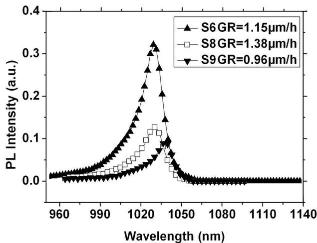
Fig. 5. PL spectra for samples prepared at different growth rates.
