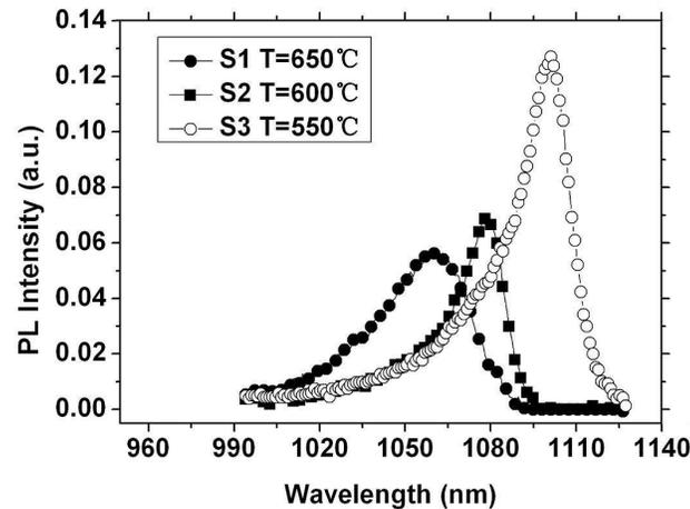
Fig. 1. PL spectrum of samples at different growth temperatures.
