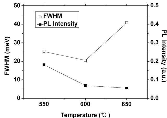
Fig. 2. PL FWHM and intensity of samples at different growth temperatures.
