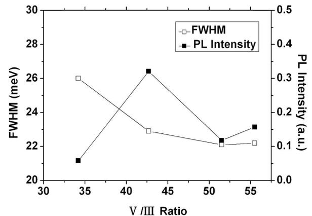
Fig. 4. PL FWHM and intensity of samples prepared at different V/III ratios.
