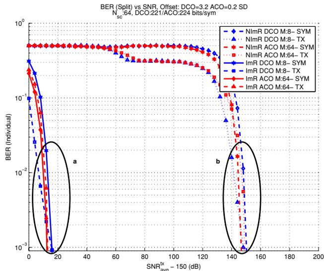
Fig. 4. Comparison of individual BER versus SNR for (a) ImR and (b) NImR.
