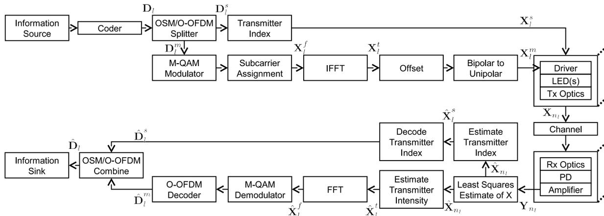
Fig. 1. Block diagram of system implementing SIS-OFDM.
