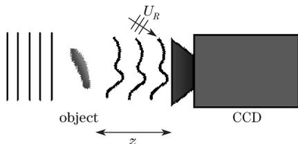
Fig. 1. Digital Holographic recording of the free space propagated field from an object illuminated by a plane wave.
