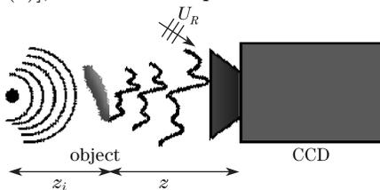
Fig. 2. Digital Holographic recording of the free space propagated field from an object illuminated by a diverging spherical wave.
