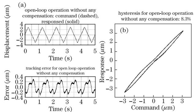
Fig. 10. Actuator response in open-loop operation without correction. (a) Desired and real outputs, and the error; (b) hysteresis curve.
