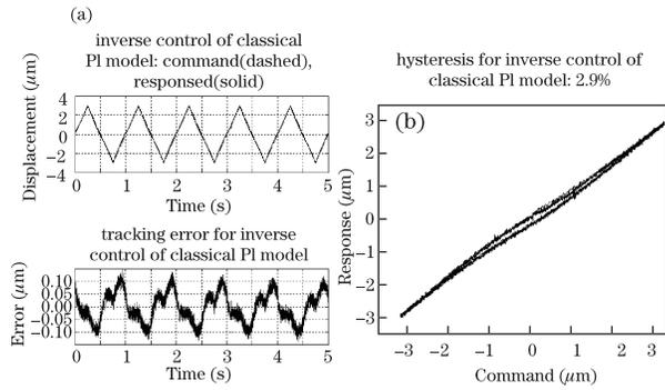
Fig. 11. Actuator response in open-loop operation with inverse controller of classical PI model. (a) Desired and real outputs, and the error; (b) hysteresis curve.
