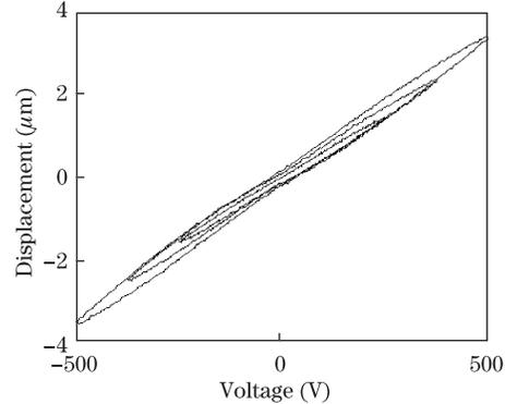
Fig. 6. Response of the modified PI model.
