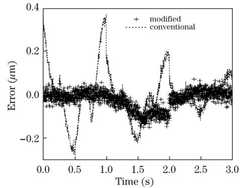
Fig. 8. Modeling errors of the conventional and modified PI models.
