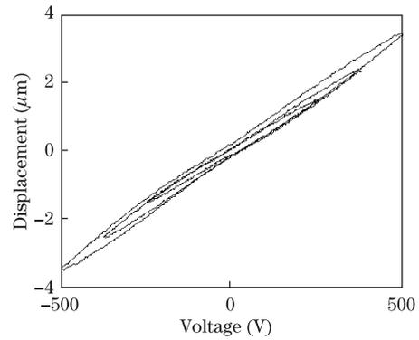
Fig. 5. Response of the piezoelectric actuator.
