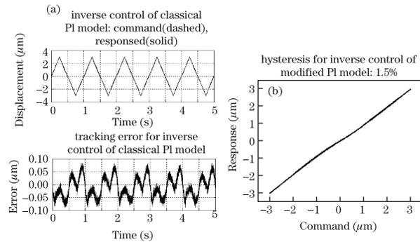
Fig. 12. Actuator response in open-loop operation with inverse controller of modified PI model. (a) Desired and real outputs, and the error; (b) hysteresis curve.
