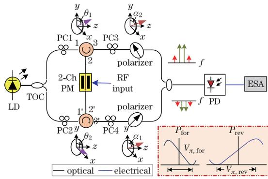
Fig. 1. Schematic of the proposed IMD3 compensation scheme. LD: laser diode; PD: photodetector; ESA: electrical signal analyzer. The inset depicts output power as a function of the applied voltage for the 2-Ch PM in opposite directions.
