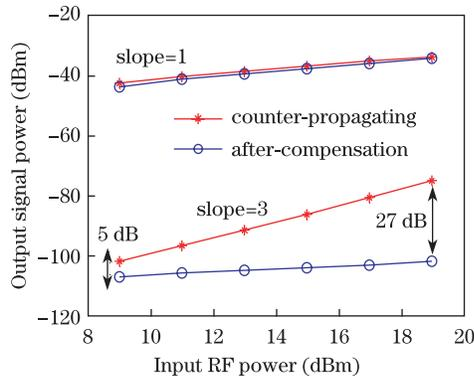
Fig. 3. Output signal power versus input RF power for counter-propagating and dispersion compensation links.
