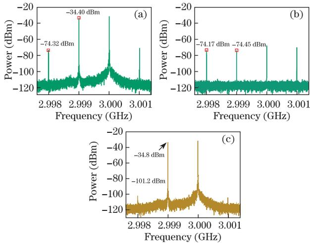
Fig. 2. Spectrum analyzer traces for the two-tone IMD3 test. (a) Counter-propagating trace; (b) co-propagating trace; (c) after the compensation of nonlinearity.
