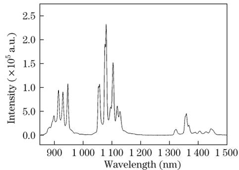
Fig. 3. Room-temperature emission spectrum of  $\text{Nd}_{0.02}\text{Y}_{1.78}\text{La}_{0.2}\text{O}_3$  ceramic.
