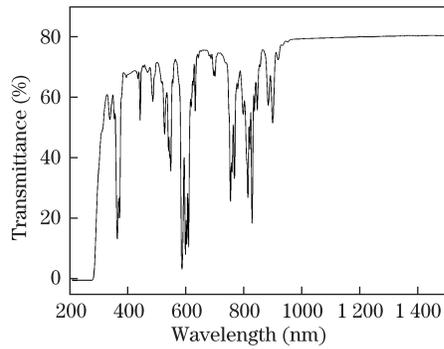
Fig. 1. Transmittance of  $\text{Nd}_{0.02}\text{Y}_{1.78}\text{La}_{0.2}\text{O}_3$  transparent ceramic.
