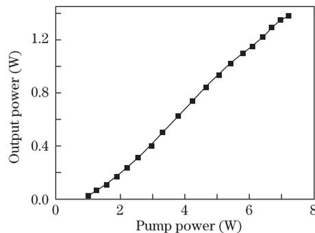
Fig. 4. The output power versus the absorbed power of  $\text{Nd}_{0.02}\text{Y}_{1.78}\text{La}_{0.2}\text{O}_3$  ceramic laser.
