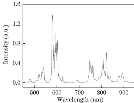
Fig. 2. Room-temperature absorption spectrum of  $\text{Nd}_{0.02}\text{Y}_{1.78}\text{La}_{0.2}\text{O}_3$  ceramic.
