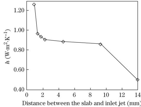
Fig. 9. Convective coefficient  $h$  as a function of distance between the Nd:glass slab and inlet jet.
