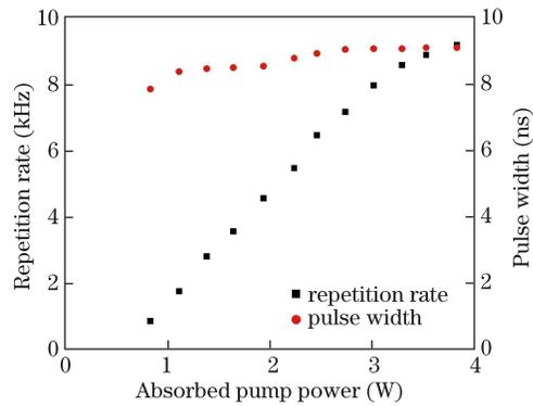
Fig. 5. Repetition rate and pulse width of Yb:YAG/Cr<sup>4+</sup>:YAG passively *Q*-switched lasers as a function of the absorbed pump power.
