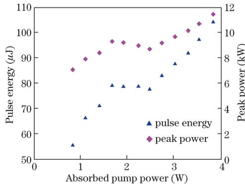
Fig. 6. Pulse energy and peak power of ceramic Yb:YAG/Cr<sup>4+</sup>:YAG passively *Q*-switched lasers as a function of the absorbed pump power.
