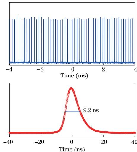
Fig. 4. Oscilloscope trace of pulse trains and laser pulse profile with pulse width of 9.2 ns, pulse energy of 83  $\mu\text{J}$ , and peak power of 9.2 kW with absorbed pump power of 2.73 W.
