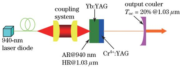
Fig. 1. Schematic diagram of laser diode pumped passively  $Q$ -switched ceramic Yb:YAG laser with  $\text{Cr}^{4+}$ :YAG as saturable absorber.
