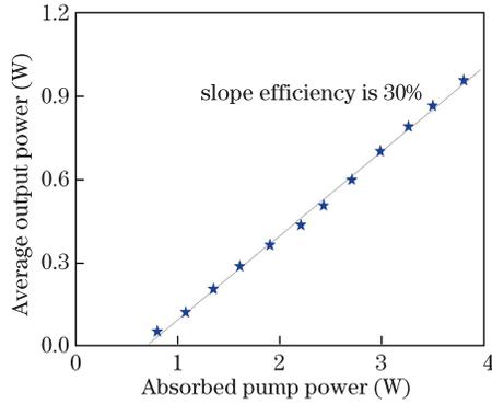
Fig. 2. Average output power of ceramic Yb:YAG/ $\text{Cr}^{4+}$ :YAG passively  $Q$ -switched lasers as a function of the absorbed pump power.
