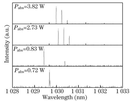
Fig. 3. Spectra of ceramic Yb:YAG/ $\text{Cr}^{4+}$ :YAG passively  $Q$ -switched lasers in different absorbed pump power levels.
