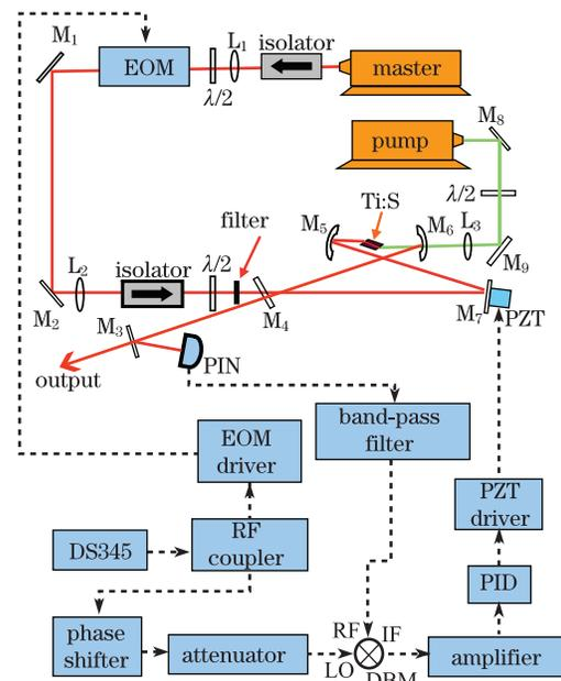
Fig. 1. Schematic of the PDH experiment in our injection-locked Ti:sapphire laser. L: lens; M: mirror; Ti:S: Ti:sapphire crystal; PZT: piezoelectric transducer; EOM: electro-optic modulator; PIN: photodiode;  $\lambda/2$ : half-wave plate; DBM: double balanced mixer; PID: proportional-integral-derivative controller; DS345: function generator; Master: master laser; and Pump: pump laser.
