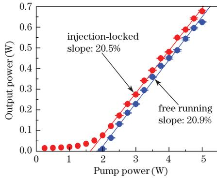
Fig. 4. Output power versus pump power during injection locking and free running.
