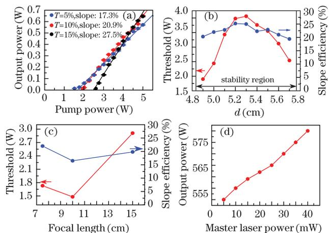
Fig. 3. (a) Influence of the different coupler transmissions on the threshold and slope efficiency; (b) threshold and slope efficiency change in the stability region; (c) influence of the focal length of the mode-matching lens for pump laser on the threshold and slope efficiency; (d) influence of the master laser power on the output power.
