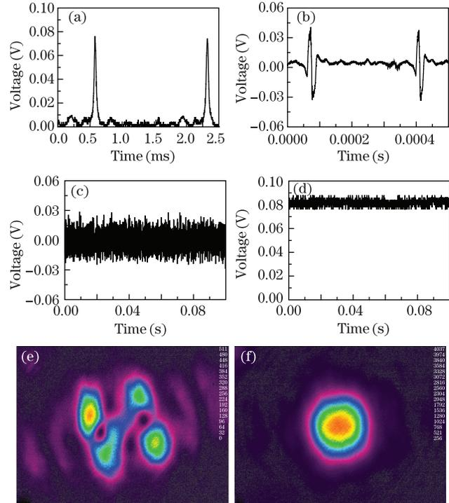
Fig. 2. (a) Transmission signal and (b) dispersive error signal during scanning; (c) error signal and (d) transmission signal after locking; laser output beam profiles when (e) unlocked and (f) locked.
