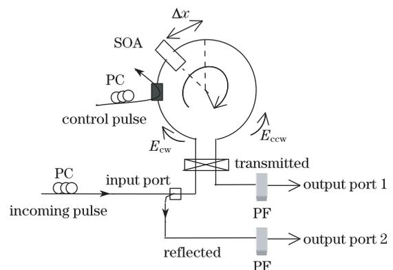
Fig. 1. TOAD-based optical switch. PC: polarization controller; PF: polarization filter;  $E_{\text{cw}}$ : clockwise electric field;  $E_{\text{ccw}}$ : counter clockwise electric field.
