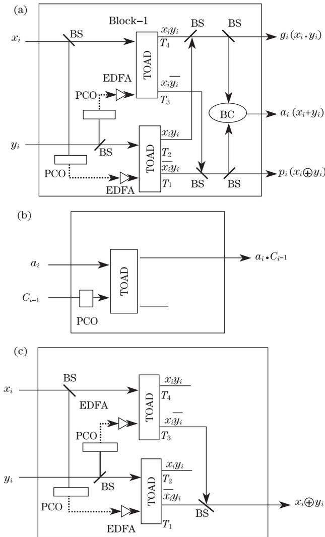
Fig. 3. (a) All-optical circuit to compute GPA; (b) all-optical AND gate; (c) all-optical XOR gate. BS: beam splitter.
