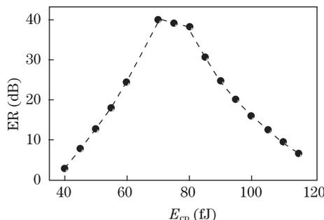
Fig. 6. Variation of ER with control pulse energy  $E_{cp}$ .
