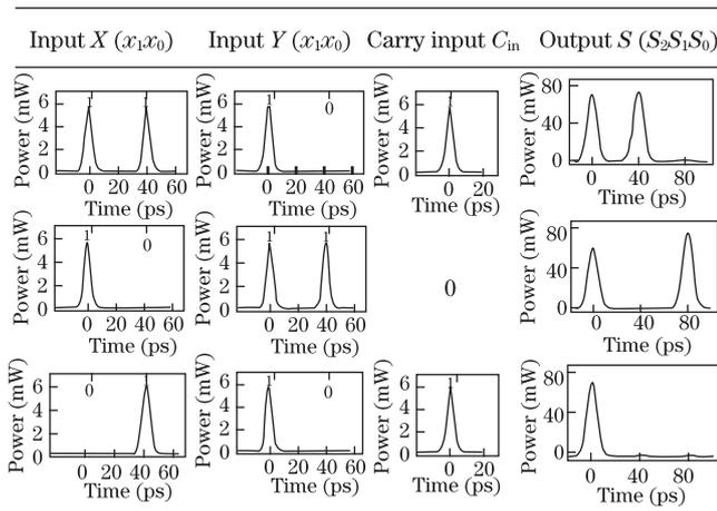
Fig. 5. Simulated waveforms of the prefix tree adder.
