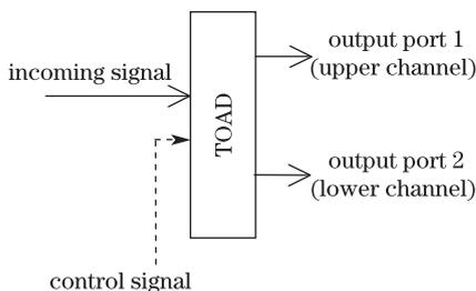
Fig. 2. Schematic diagram of TOAD-based optical switch.
