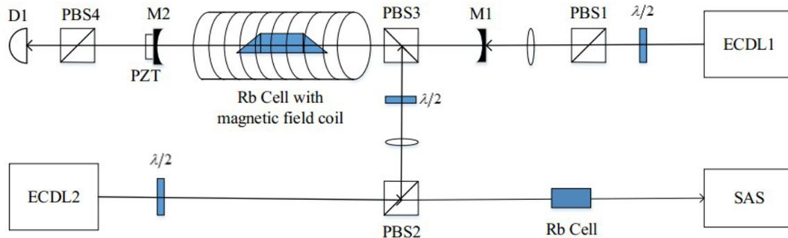
Fig. 2. Experimental setup: D1 and D2, detectors;  $\lambda/2$ , half-wave plate.
