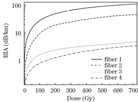
Fig. 2. Growth of the RIA at 1310 nm in four types of fibers during irradiation.
