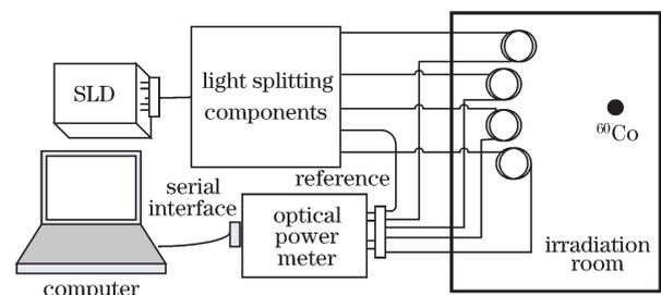
Fig. 1. Experimental setup for measuring the RIA in PM fibers.
