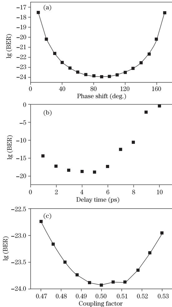
Fig. 7. Measured sensitivity curves versus (a) phase shift, (b) delay time, and (c) coupling factor.
