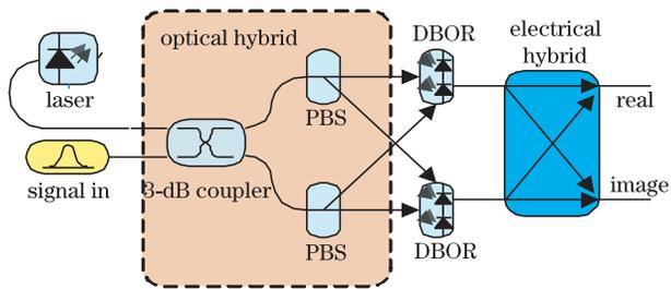
Fig. 1. Principle of IRR.
