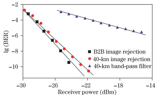
Fig. 5. Measured BER curves versus received downstream power. B2B: back-to-back.
