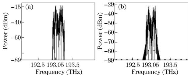
Fig. 3. Measured optical spectra for (a) 40-Gb/s FSK signal and (b) 2.5-Gb/s ASK signal.
