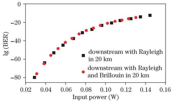
Fig. 6. Measured BER curves versus input power.
