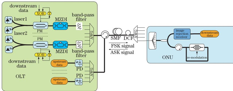
Fig. 2. Schematic for orthogonal FSK/ASK re-modulation in WDM-PON using image rejection. PD: photodetector; SMF: single-mode fiber; DCF: dispersion compensating fiber.
