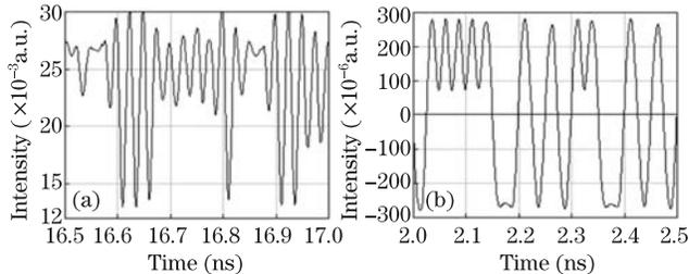
Fig. 4. Measured waveforms for (a) band-pass filter and (b) image rejection.
