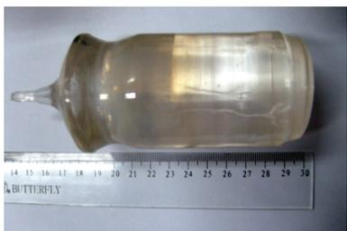
Fig. 1.  $\text{LiAlO}_2\text{:Mn}$  single crystal grown by the CZ pulling method.
