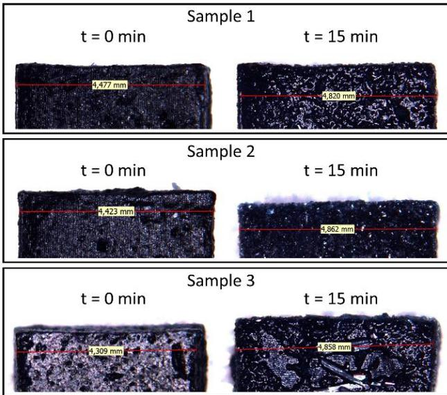
**Figure 2** Swelling tests in electroplating electrolyte solution.
