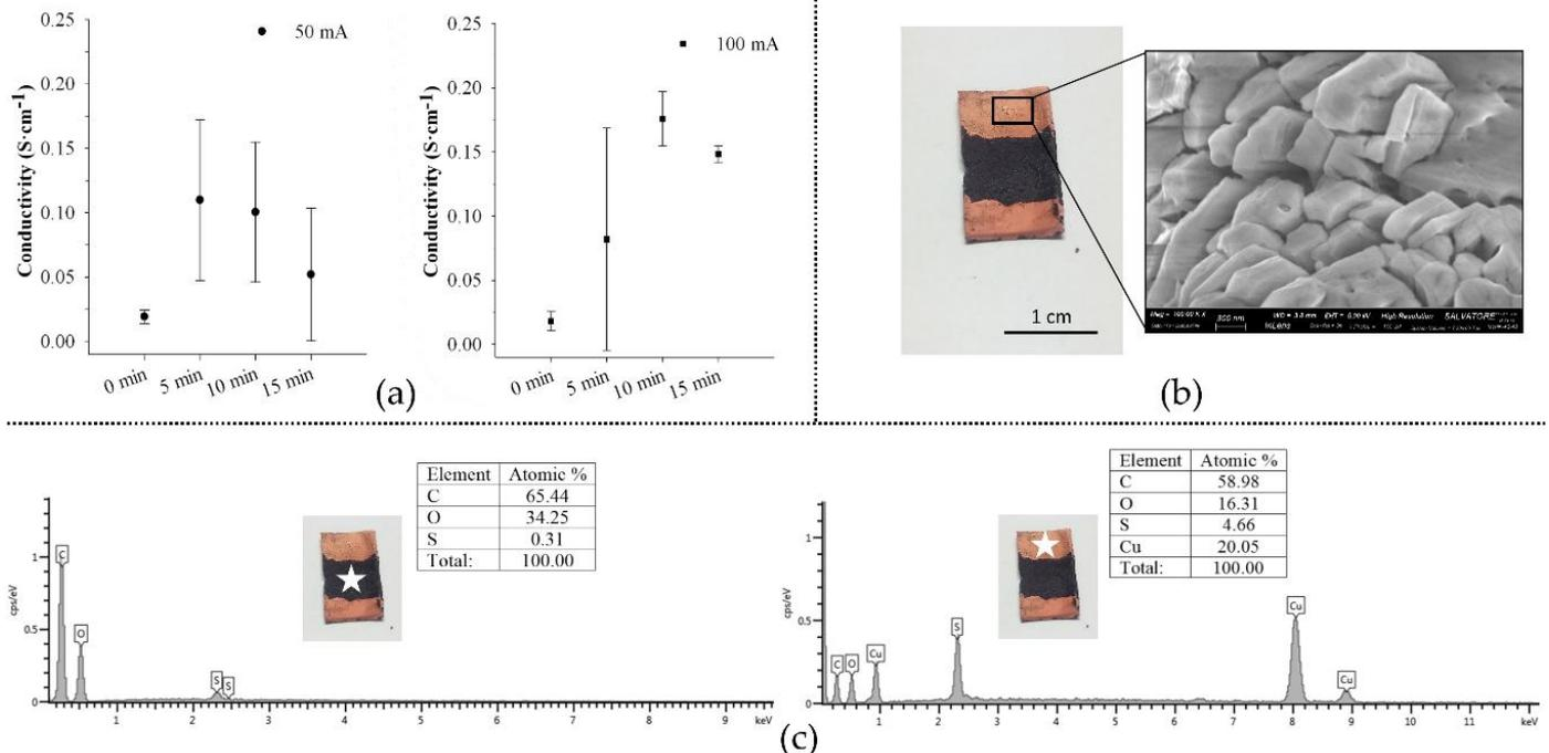
**Figure 3** Characterization of 3D printed Cu electroplated PEGDA/PEDOT samples. (a) Electrical characterization results for samples deposited with Cu electrodeposition at 50 mA and 100 mA. (b) A sample electroplated (left) with the optimized parameters (100 mA nominal current for 15 min) and a FESEM image showing the typical Cu grains. (c) Atomic composition of
