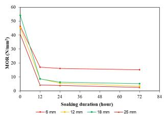
Fig. 2: Effect of soaking duration on the MOR of MDF at various board thickness
