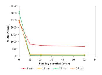
Fig. 1: Effect of soaking duration on the MOE of MDF at various board thickness
