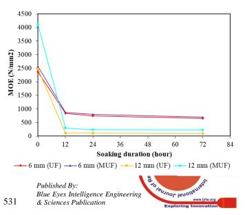
Fig. 3: Effect of soaking duration on the MOE of MDF bonded with different resin.
