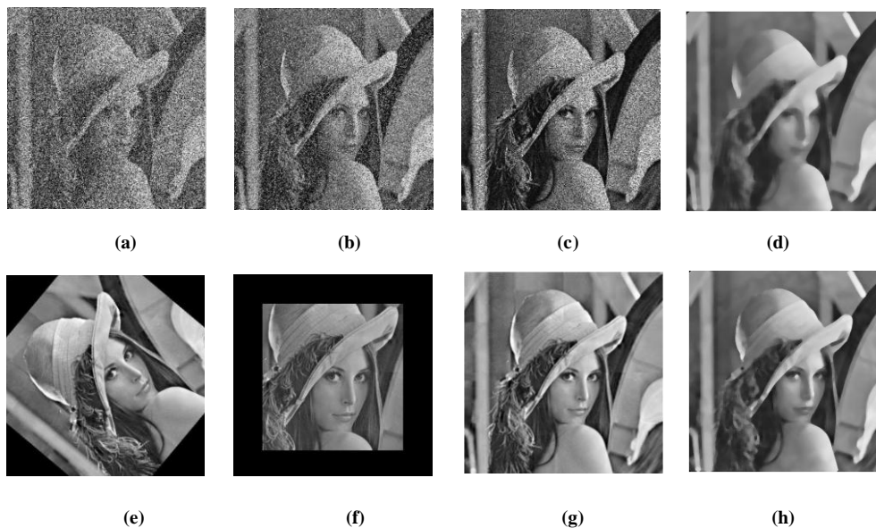
Fig.7. Watermarked Images After applying attacks (a) Gaussian Noise (M=0,V=0.5) (b) Salt and Pepper Noise (0.4) (c) Speckle Noise(0.4) (d) Median filtering (7x7) (e) Rotation (f) Cropping (g) Resizing (512-256-512) (h) Compression
