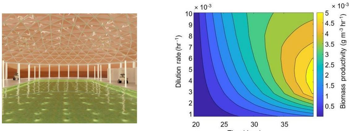
Figure 3. Render of a possible open pond on a Martian dome (a) and simulated effect of the cultivation of *S. platensis* on Mars in the pond fed-batch mode.
