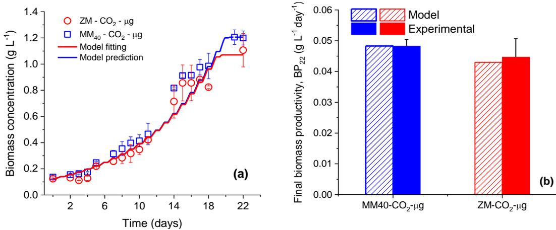
Figure 1: Comparison between experimental and model results in terms of biomass concentration evolution (a) and biomass batch productivity after 22 days (b).
