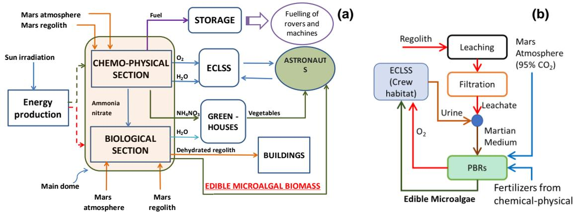
Figure 1. Scheme of the ISRU process to produce useful materials on Mars (a) and focus on the production of microalgae in the biological section (b). Part (a) of the Figure is adapted from Concas et al. (2012).
