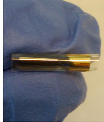
Figure 4: A wrapped "capsule" made of the THz metamaterials patterned on silk films.
