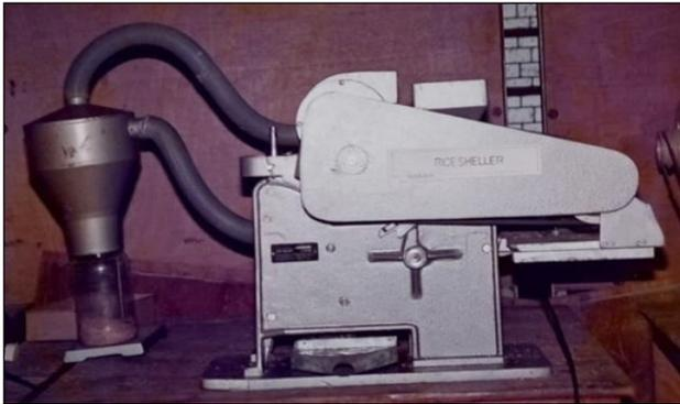
**Plate 1:** Rubber Roll Sheller (Lab Model)
