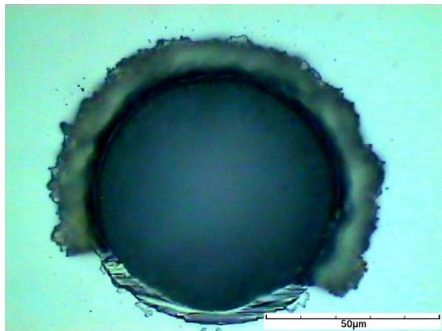
Figure 12: Hole drilled using a long pulse laser
