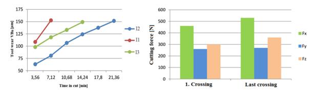
Fig. 3. (a) The dependence of the tool wear on the time in cut; (b) Cutting forces
