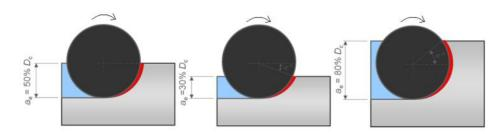
Fig. 2. Description of radial immersion [4]
