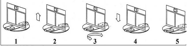
Fig. 2. Automatic Pallet Changer Operation Sequence
