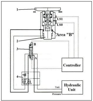
Fig. 4. Automatic Pallet Changer Arm Down Mechanism
