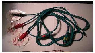
Fig. 2. EKG electrodes and shielded cable
