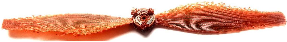
Fig. 15. Prototype of 3D printed propeller
