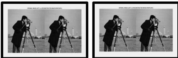
Figure. 14 Reconstructed images by feeding the DCT coefficients to the inverse DCT: (a) retaining 50% of the coefficients, and (b) retaining 25% of the coefficients
