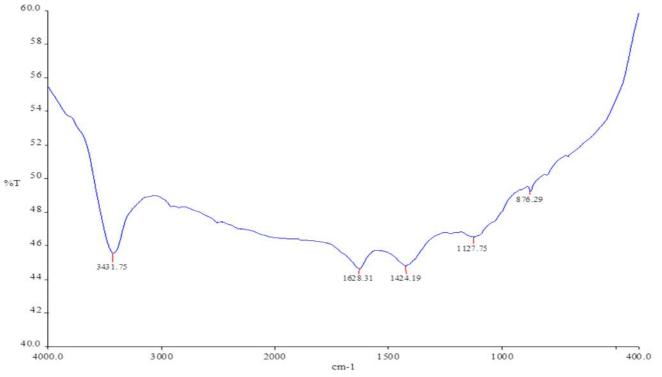
The FT-IR absorption spectrum of the sample Mansolai after purification reveals that the IR absorption peak at 1420.18 cm-1 due to presence of S=O functional group stretching. Vibrational peak at 3409.68 cm-1 maybe due to the presence of primary
