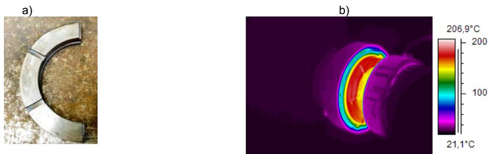
**Fig. 4.** Brake disc (a) and its thermal image on a test stand (b)
