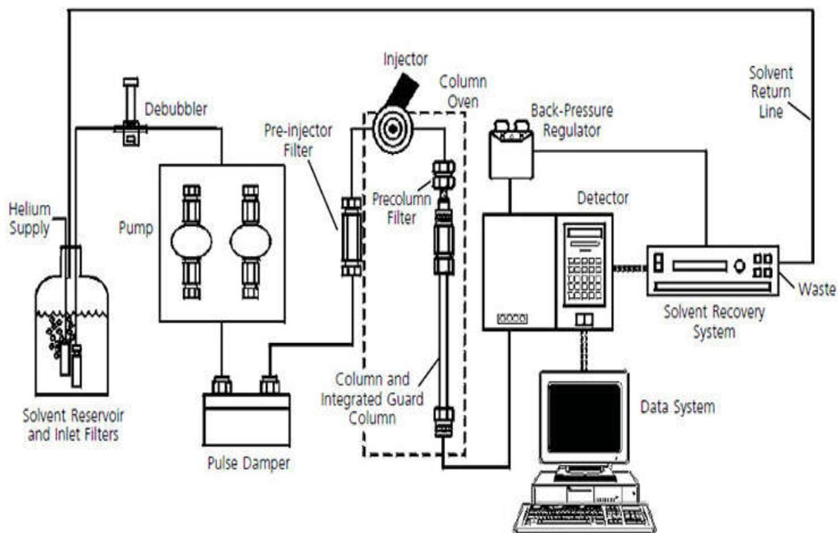
**Figure 1: Block diagram of UPLC System**
