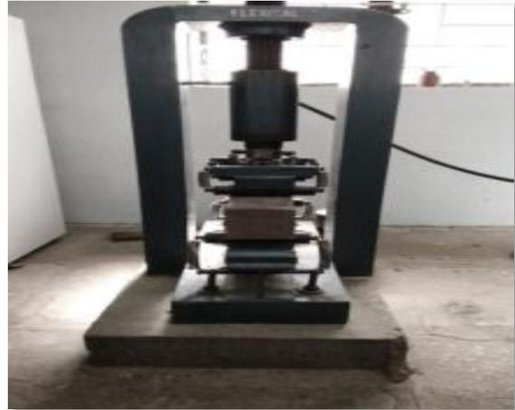
**Figure 5** Prism subjected to third point loading method
