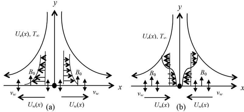
FIGURE 1. Physical model and coordinate system: (a) Stretching sheet and (b) Shrinking sheet
