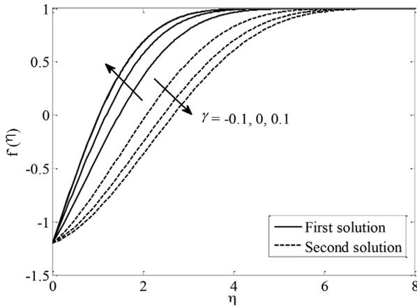
FIGURE 6. The velocity profiles  $f'(\eta)$  for different values of  $\gamma$  when  $M = 0.001$  and  $\varepsilon = 1.2$  (shrinking case)
