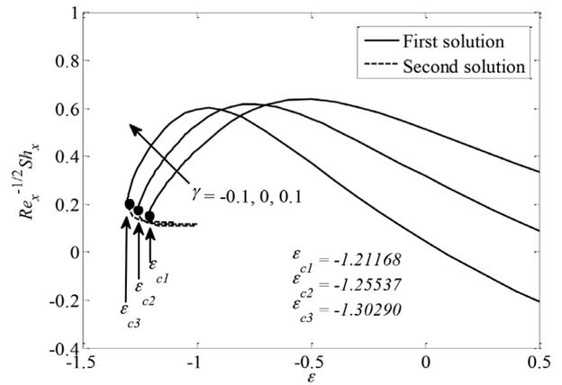
FIGURE 4. Variation of the local Sherwood number  $Re_x^{-1/2} Sh_x$  with  $\epsilon$  for different values of  $\gamma$  when  $Pr = 7, M = 0.01, Nb = 0.1, Nt = 0.1, Le = 1, Cr = 0.1$  and  $Sr = 1$
