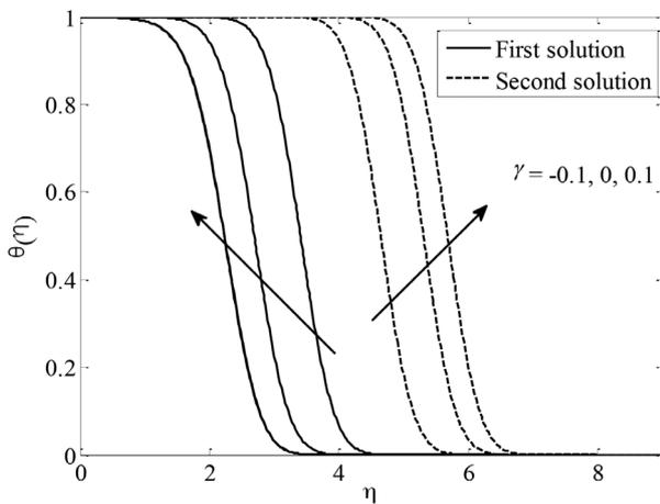
FIGURE 7. The temperature profiles  $\theta(\eta)$  for different values of  $\gamma$  when  $Pr = 7, M = 0.01, Nb = 0.1, Nt = 0.1, Le = 1, Cr = 0.1, Sr = 1$  and  $\varepsilon = 1.2$  (shrinking case)
