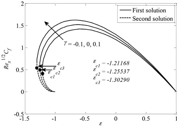
FIGURE 2. Variation of the skin friction coefficient  $Re_x^{-1/2} C_f$  with  $\epsilon$  for different values of  $\gamma$  when  $M = 0.01$
