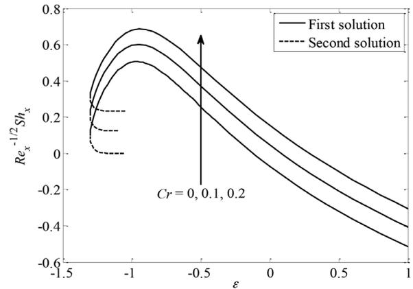
FIGURE 5. Variation of the local Sherwood number  $Re_x^{-1/2} Sh_x$  with  $\epsilon$  for different values of  $Cr$  when  $Pr = 7, M = 0.01, Nb = 0.1, Nt = 0.1, Le = 1, \gamma = 0.1$  and  $Sr = 1$
