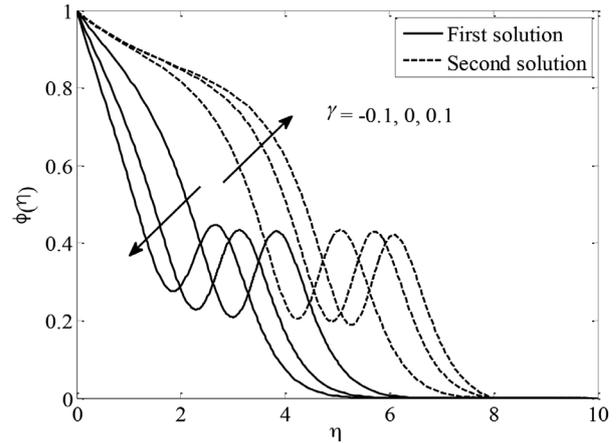
FIGURE 8. The concentration profiles  $\phi(\eta)$  for different values of  $\gamma$  when  $Pr = 7, M = 0.01, Nb = 0.1, Nt = 0.1, Le = 1, Cr = 0.1, Sr = 1$  and  $\varepsilon = 1.2$  (shrinking case)
