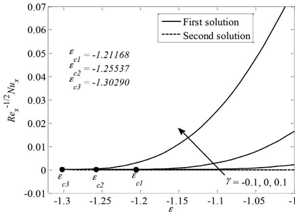
FIGURE 3. Variation of the local Nusselt number  $Re_x^{-1/2} Nu_x$  with  $\epsilon$  for different values of  $\gamma$  when  $Pr = 7, M = 0.01, Nb = 0.1, Nt = 0.1, Le = 1, Cr = 0.1$  and  $Sr = 1$
