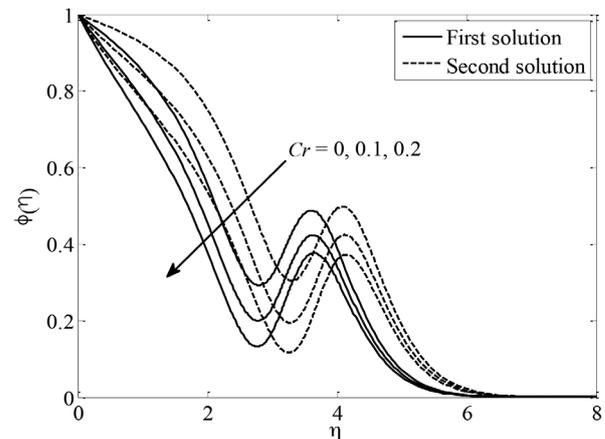
FIGURE 9. The concentration profiles  $\phi(\eta)$  for different values of  $Cr$  when  $Pr = 7, M = 0.01, Nb = 0.1, Nt = 0.1, Le = 1, \gamma = 0.1, Sr = 1$  and  $\varepsilon = 1.3$  (shrinking case)
