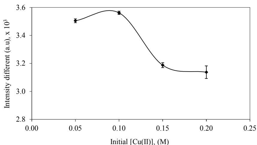
FIGURE 3. Effects of immobilized Cu(II) concentration on glutamate response at 691 nm ([Glu] = 2 M)
