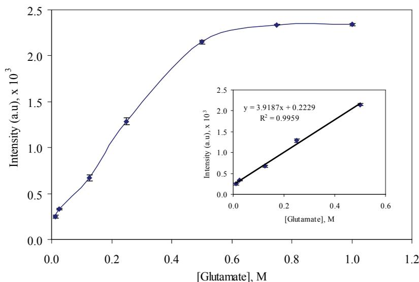
FIGURE 6. Dynamic range of the glutamate sensor response to various concentrations of glutamate determined at 691 nm. The linear range is also shown in the inset
