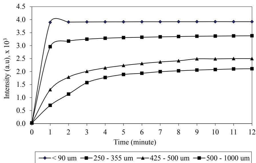
FIGURE 5. Glutamate sensor response at 691 nm at different size of sol-gel/Cu(II)
