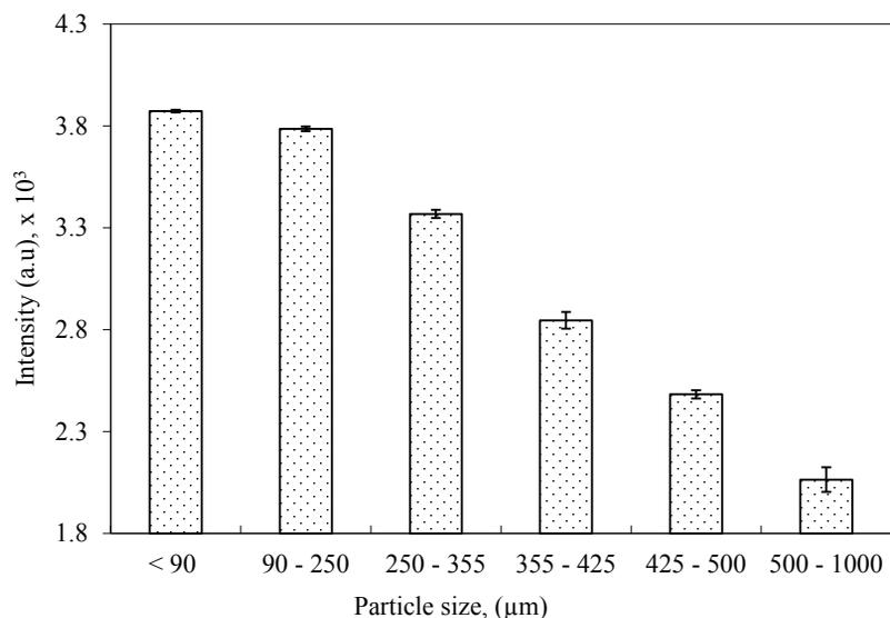
FIGURE 4. Effects of sol-gel particle size on glutamate sensor response at 691 nm
