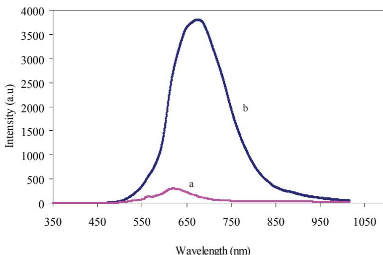
FIGURE 2. Reflectance spectra for immobilized copper (II) ions: (a) before and (b) after reaction with 2 M glutamate
